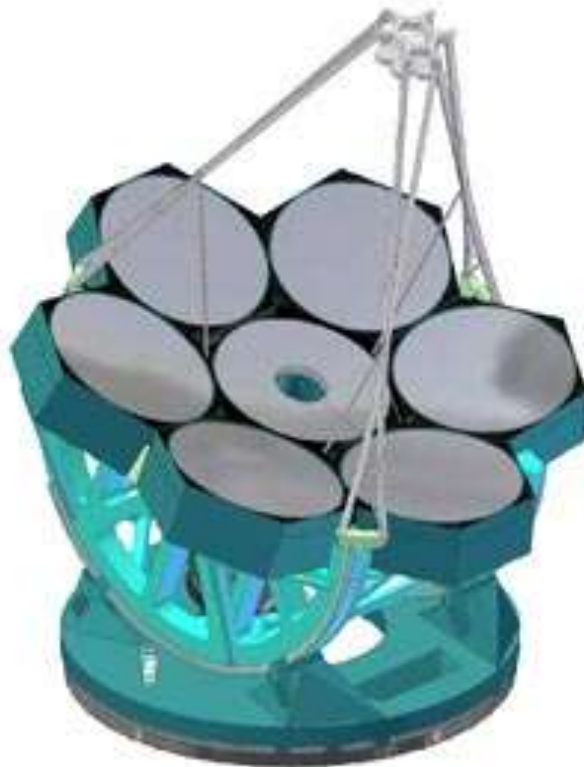
Mirror arrangement of the Giant Magellan Telescope
