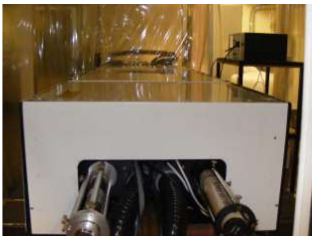
The solid-state laser that fires its beam up through the central column to the dome above
