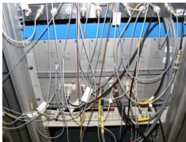
The air-radar control panel that cuts the laser if an aircraft is detected
